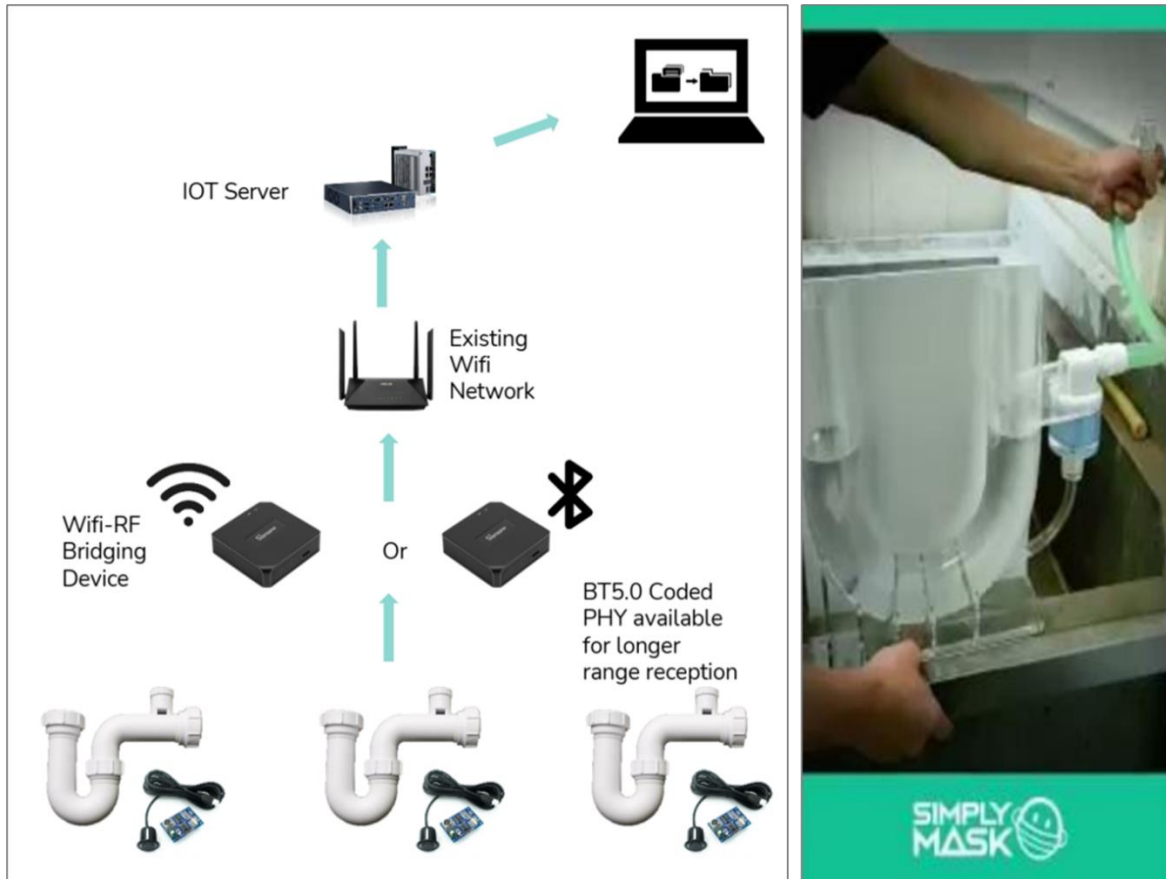
Figure 1 Smart ESG U-traps: U-Trap + Internet of Things (IoT) Solution in anti-pandemic control
